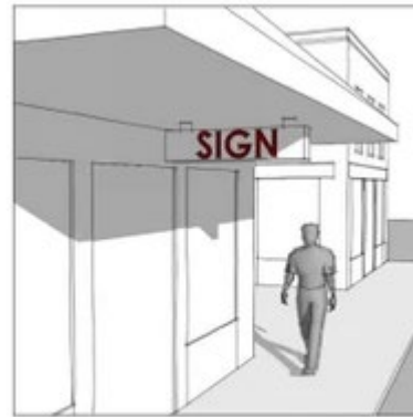
Figure – Suspended Sign
