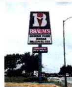
Sign support wrapped in masonry
